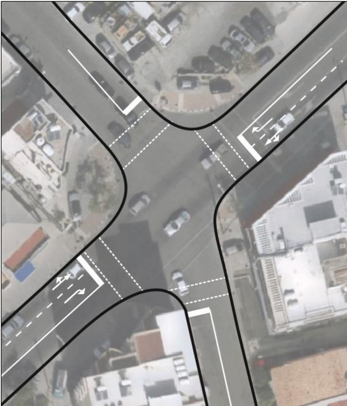
Figure A-VII 4: Accident Accumulation Zone 4: compact intersection design, picture: © Google earth
