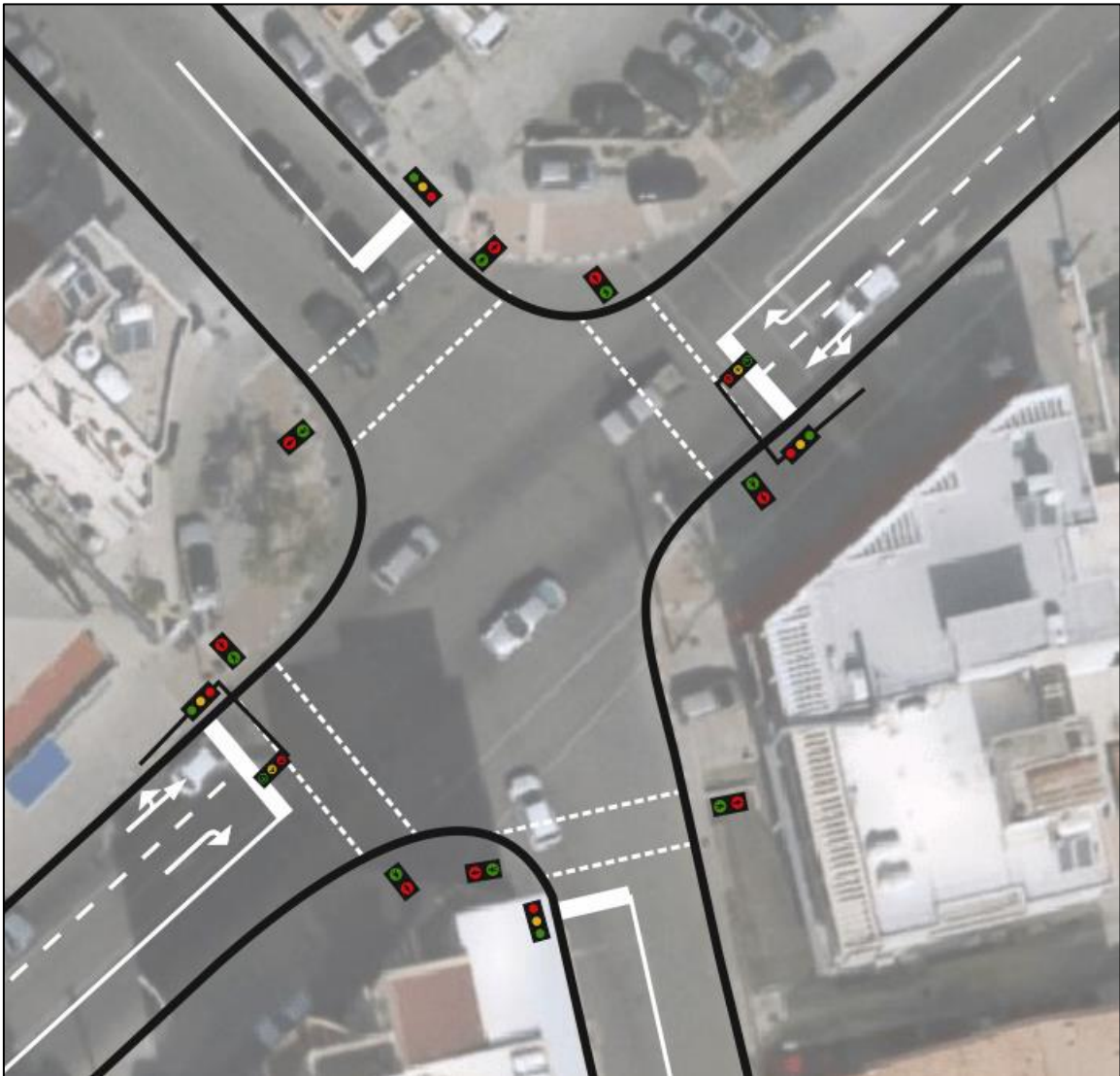
Figure A-VII 6: Accident Accumulation Zone 4: signalisation of right turns and markings, picture: © Google earth
